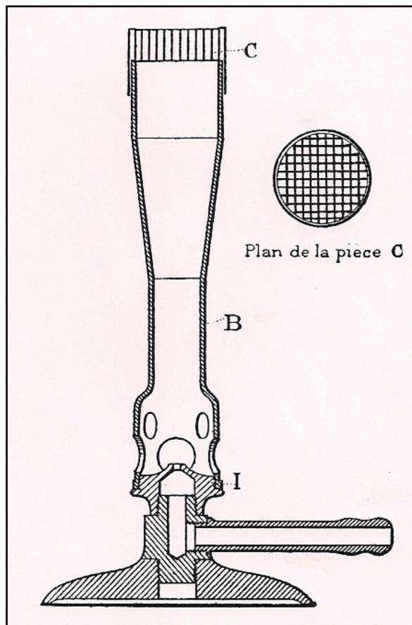
Figure 1. A cross-section of Meker's original burner (2).
