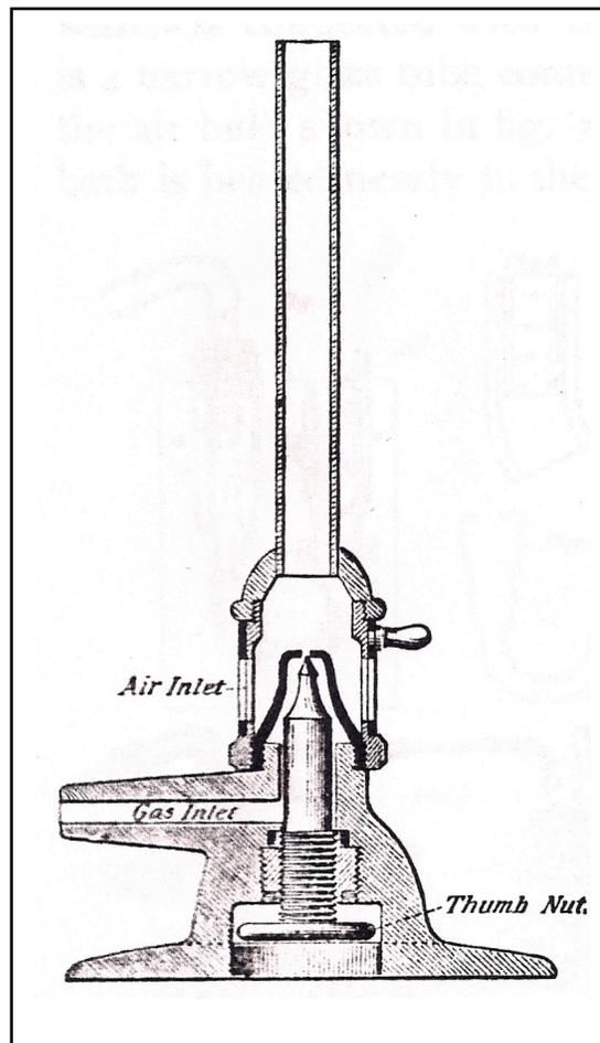
Figure 2. A cross-section of Venable's original burner (4).
